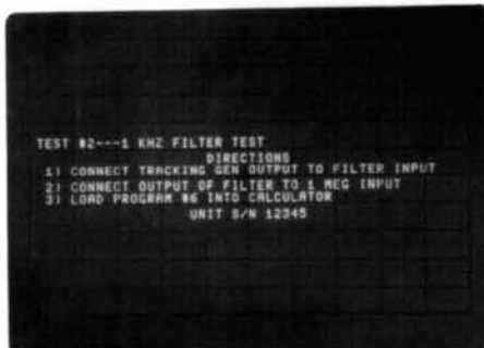
HP 3585A displays detailed instructions for an automatic filter test downloaded from an external computer.
